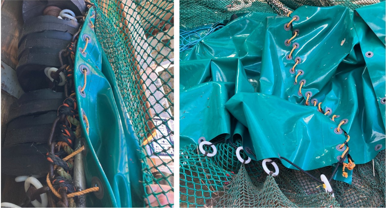
Figure 19 : The front part of the sediment sheet was attached into the ground gear and to the bottom panel with plastic rings and elastic rope.
