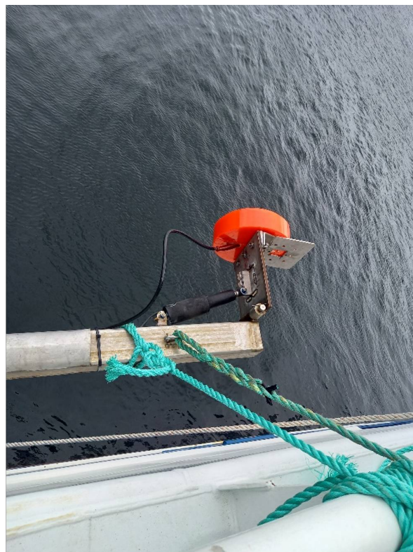
Figure 3. Detail of the pole and the transducer off the water during cruising. The transducer is mounted in a plate that is tilted by a hydraulic piston.
