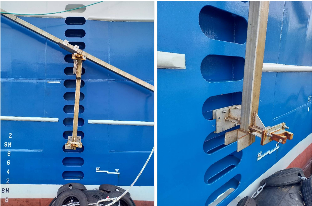
Figure 2. Mounting of pole to starboard side of FV Libas.
