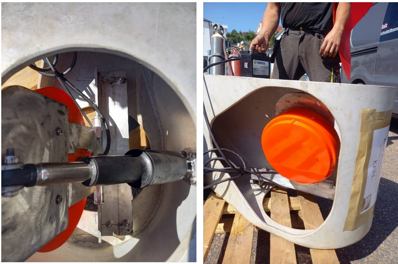
Figure 5. Detail of the hydraulic piston that will provide with tilt for the transducer (left) and transducer inside the blister (right).
