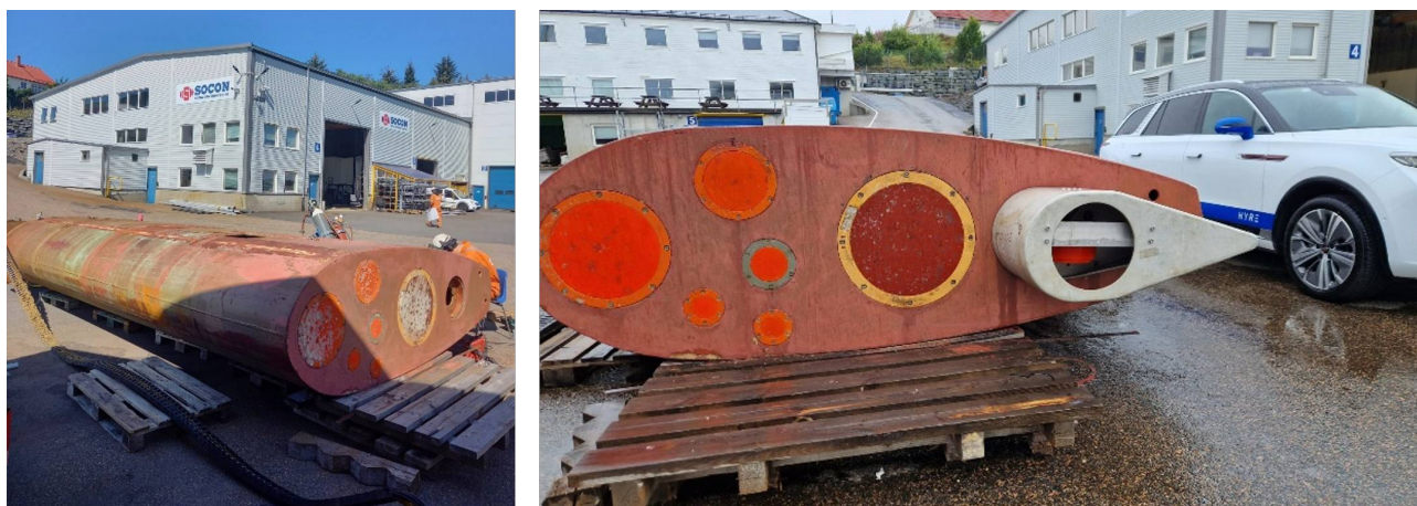
Figure 4. Drop keel from FV Libas with transducers mounted in the bottom, with cable chain along the left side of the keel (left). Aluminum blister containing the ES200-3C transducer when mounted (right).
