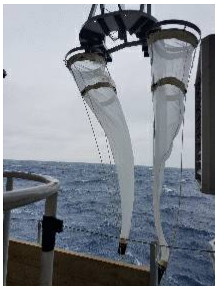
Figure 3.2. The WP2 DUO deployment from the CTD hangar of RV Kronprins Haakon 14 March 2019. Foto: Tone Falkenhaug, IMR.
