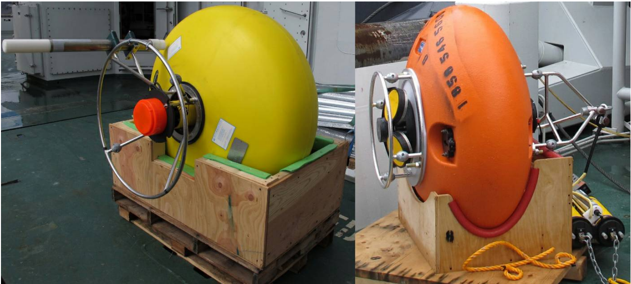
Figure 15.1. Left: a Simrad WBAT echosounder mooring ready for deployment. The orange disc is the acoustic transducer, the yellow cylinder (mostly obscured) is the WBAT echosounder, the yellow eelipsoid the flotation, and the white/silver tube an ARGOS tracker. Right: A Nortek Signature100 echosounder mooring ready for deployment. The echosounder transducer is the black disk to the left, and the yellow discs the ADCP transducers.
