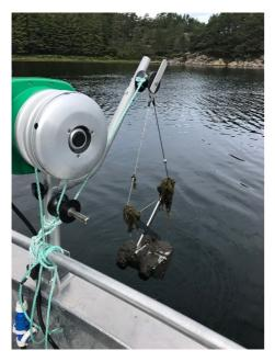
Figure 2. Van Veen Grab sediment sampler.
