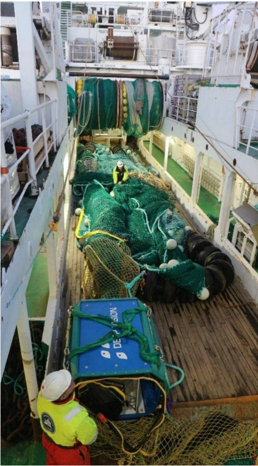
Figure 5 . The Selstad trawl and DV are prepared for deployment.
