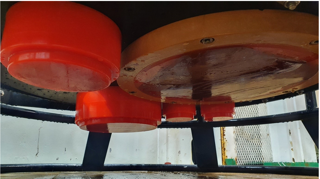
Figure 16 .2. Acoustics-equipped probe ('TS-probe') as suspended by a reinforced electric-optic wire for live communication and data viewing. TS-probe contains four broadband transceivers (black cylinder in the middle) that are coupled to the transducers mounted on a motorized plate (bottom). Probe was operated at 100-300 m depth (Image credit: Rokas Kubilius/Institute of Marine Research).
