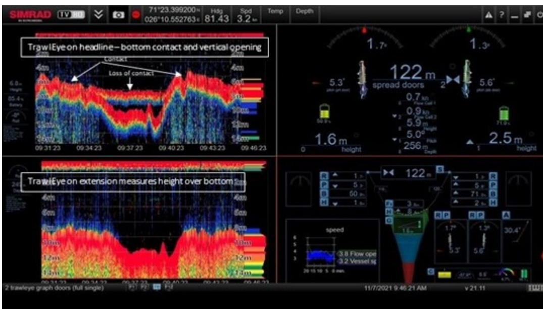
Figure 6 . Screen shot from TV80 (KM) software. Showing the TrawlEye echograms (bottom contact and height over seabed) and data from door and flow sensors on the rig.
