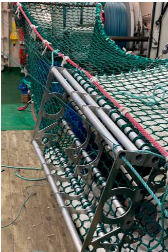
Figure 6. Deep Vision, Fishery frame and rubber sheet attached with 7-meter 155 mm square mesh extension.
