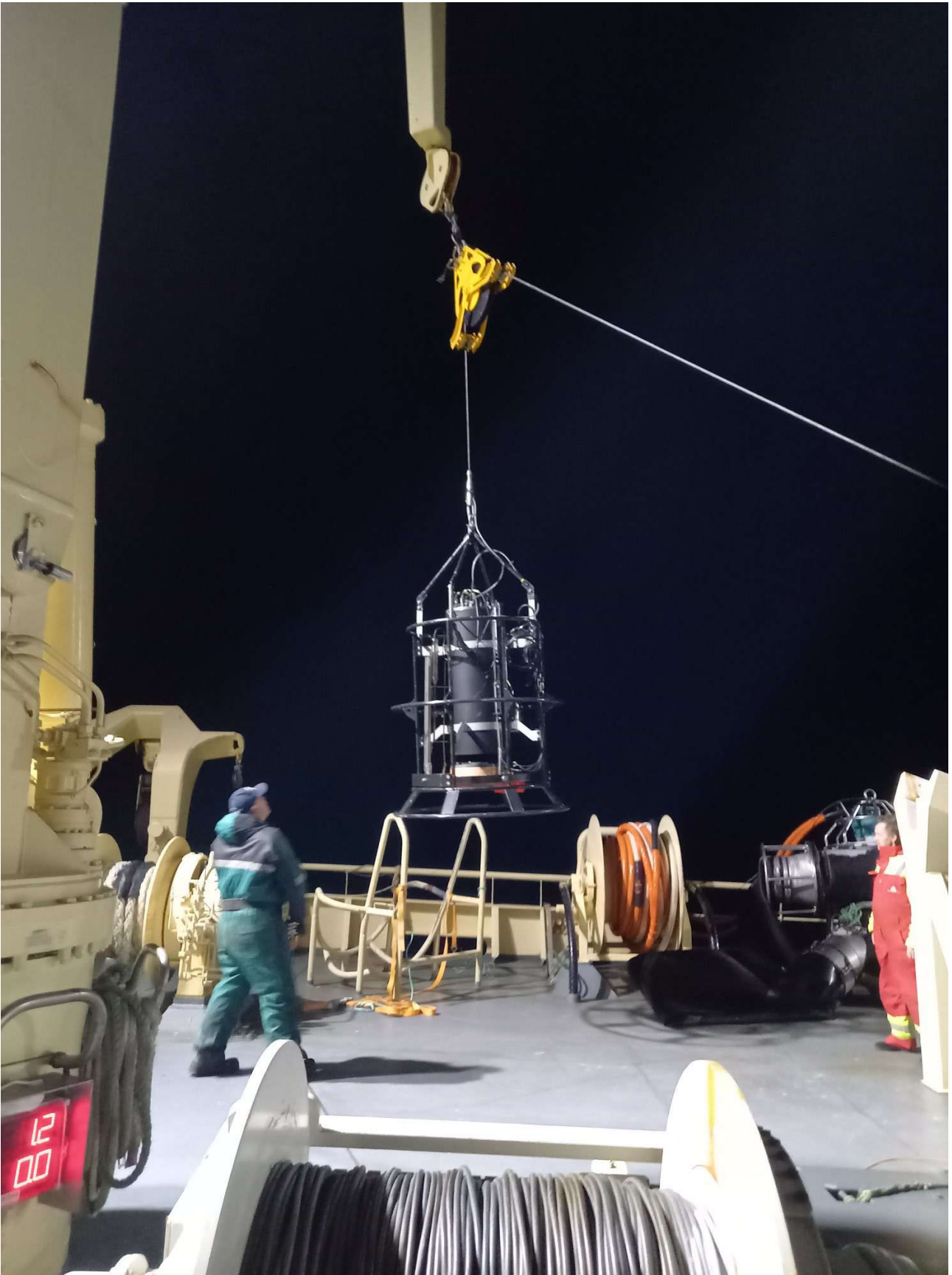
Fig. 11 . Retrieval of the TS probe onboard Eros after data collection for single fish target strength measurements.
