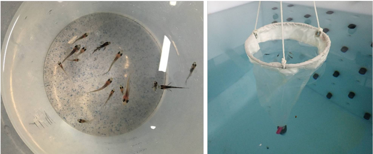
Figure 4. Left: Haddock juvenile before testing. Right: Haddock juveniles were placed in a plankton net in the EMSS tank for exposure to the different electromagnetic fields.
