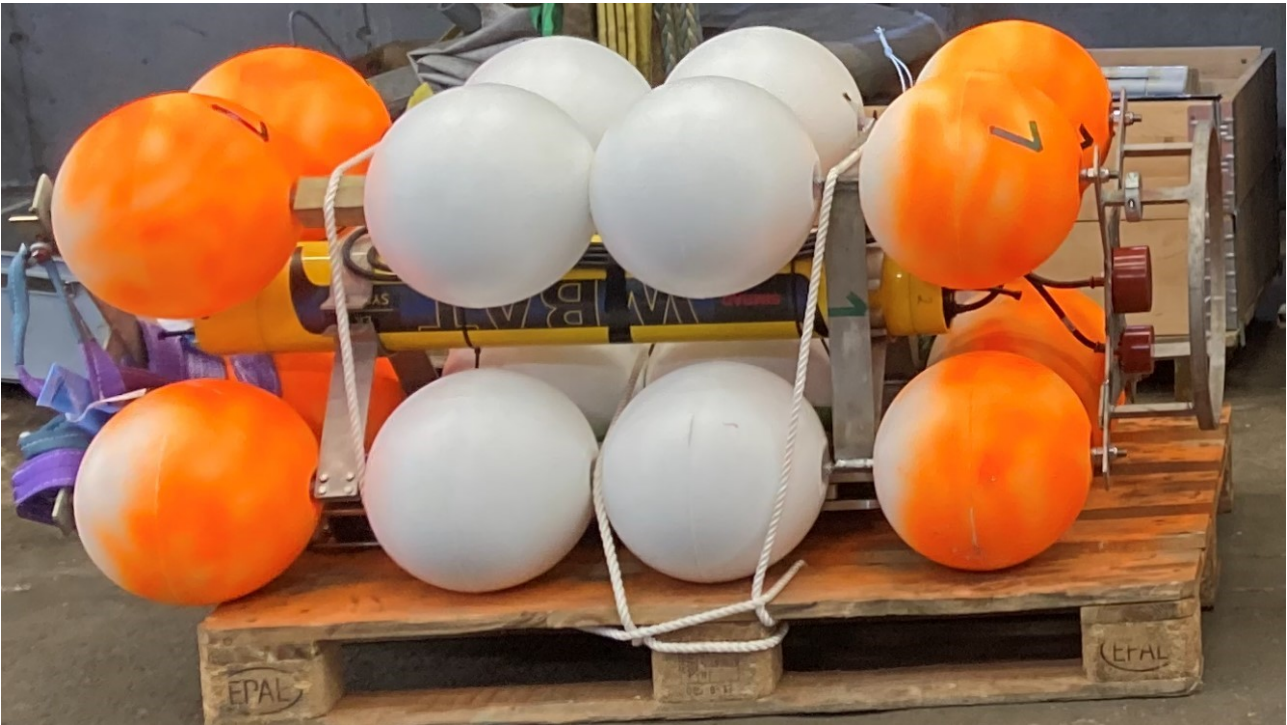
Figure 3. WBAT (wide band transceiver) with two upwards looking transducers. Picture by Anne Christine Utne Palm.
