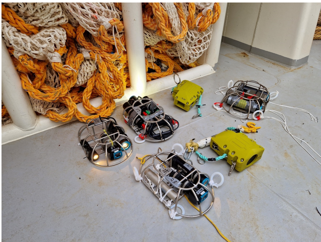
Figure A1 – various camera systems and other instruments ready for deployment before Test haul #T2: top left, GoPro cameras (in a B-group housing) in a protective steel “dome-frame”, with two white lights; top centre a FossTech Codend Choker Unit (CCU); top right, the “DarkVision” camera system in a “dome-frame”; centre right, a removal depth sensor and backup CCU; and bottom centre, a GoPro Hero 5 (in a B-group housing) in a “dome-frame”, with one white light and a depth sensor, for monitoring the CCU opening time and depth.
