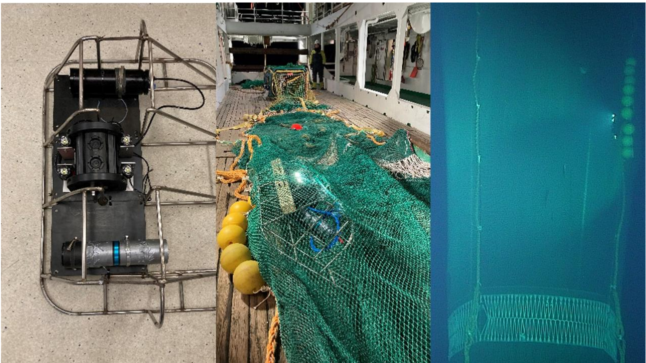
Figure 12. Fisheries Deep Vision system. Left: frame with camera and lighting system. Centre: mounting inside trawl (middle of last section of 40 mm mesh). Right: image from FOCUS towed vehicle during trawling.
