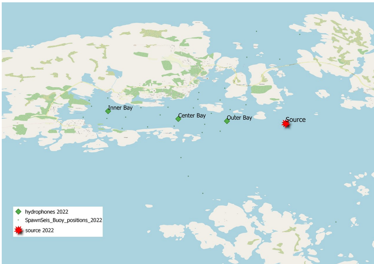
Figure 2. Positions for the source ship (red double star) and the three hydrophones (green diamonds) and the telemetry receivers (green small dots) in the experimental bay in Bakkasundet, Austevoll.
