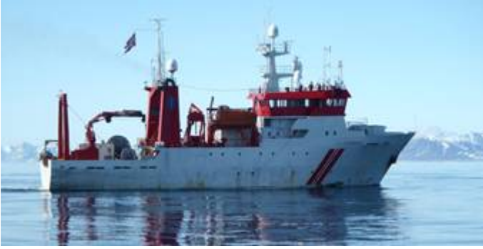
Figure 3. RV H.U Sverdrup II. Length: 55 m; max speed 15 knots; crew: 7
