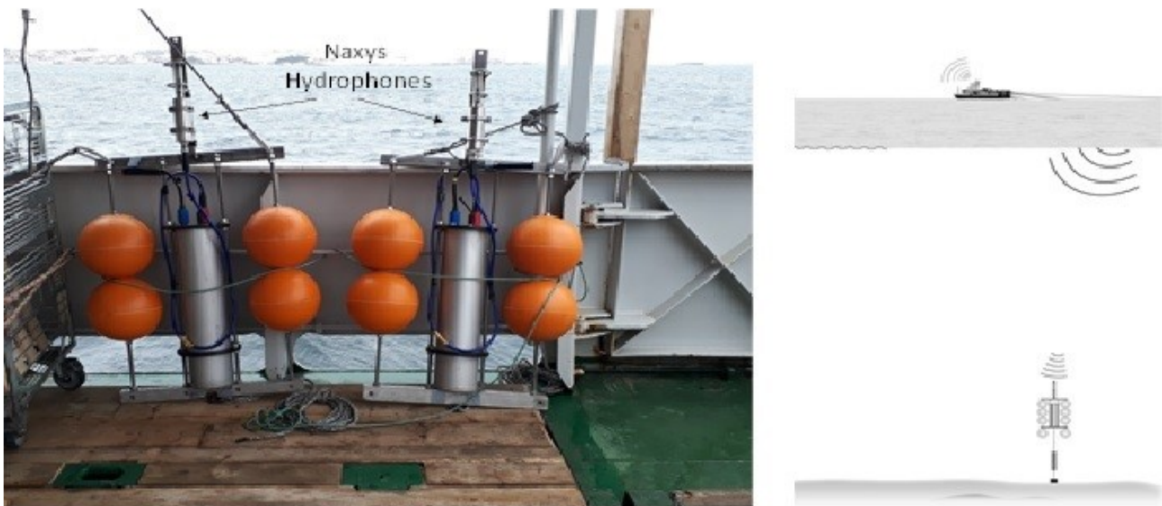
Figure 6. The two hydrophone platforms onboard HUS, ready to be deployed (left) and a figure of how it looks when deployed (right).
