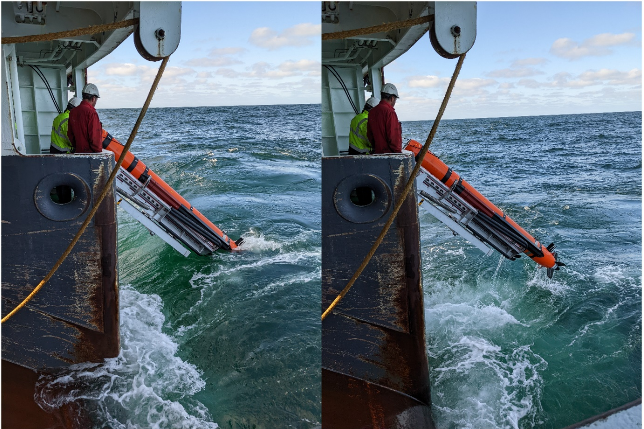
Launching the AUV into large swell - borderline conditions for AUV launch. Photo R Ross
