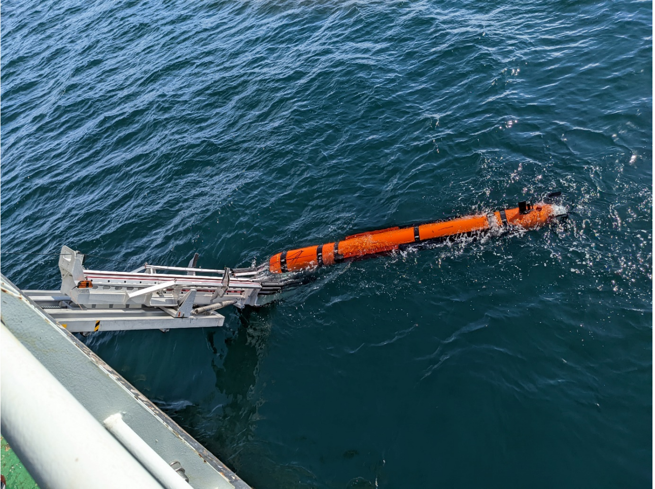
AUV leaving the stinger viewed from the deck above. Photo R Ross
