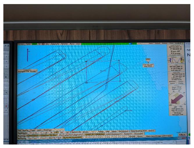
Olex screen showing planned SBP lines and the square around AUV34
