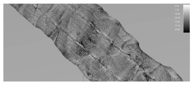
Example NGU processed backscatter data (FMGT) from AUVMøre\_VL1293 (Mission 55 20220606) showing along track striping (sector problems?)
