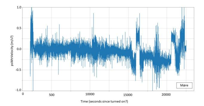
Above plot is psWtrVelocity – psBtmVelocity (i.e. residual currents in the cross AUV direction). Again the magnitude of the current is plausible. The AUV descended the slope at an angle, so we would expect the slope current to be split between along- and across-AUV directions.
