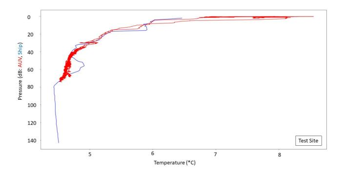
Comparison between shipborne and AUV temperature. The shipborne CTD was taken in a deeper area slightly off the site. Overall, the match is reasonable in the upper part of the water column. The feature in the shipborne CTD at 45-70m is not reproduced in the temperature profile either, but more resembles the AUV conductivity profile above. While the cause is unknown, it lends support to the hypothesis that the water properties really are different in the shallow and deeper areas.
