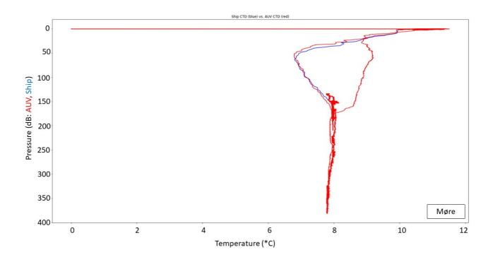
Comparison between ship and AUV temperature. The downcasts follow each other well, but it is possible that there is a small offset of some kind. It is also possible the difference is due to natural variation and a (small) difference in position and time of the two casts.
