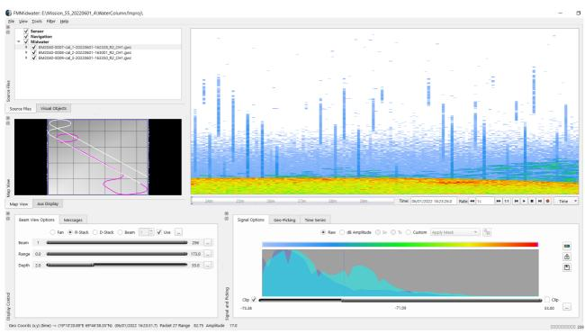
Example data from test area Tromsø – noise appears as vertical striping.
