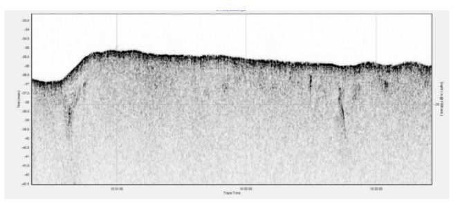
Example sub bottom profiler data from AUVMøre VL1071
