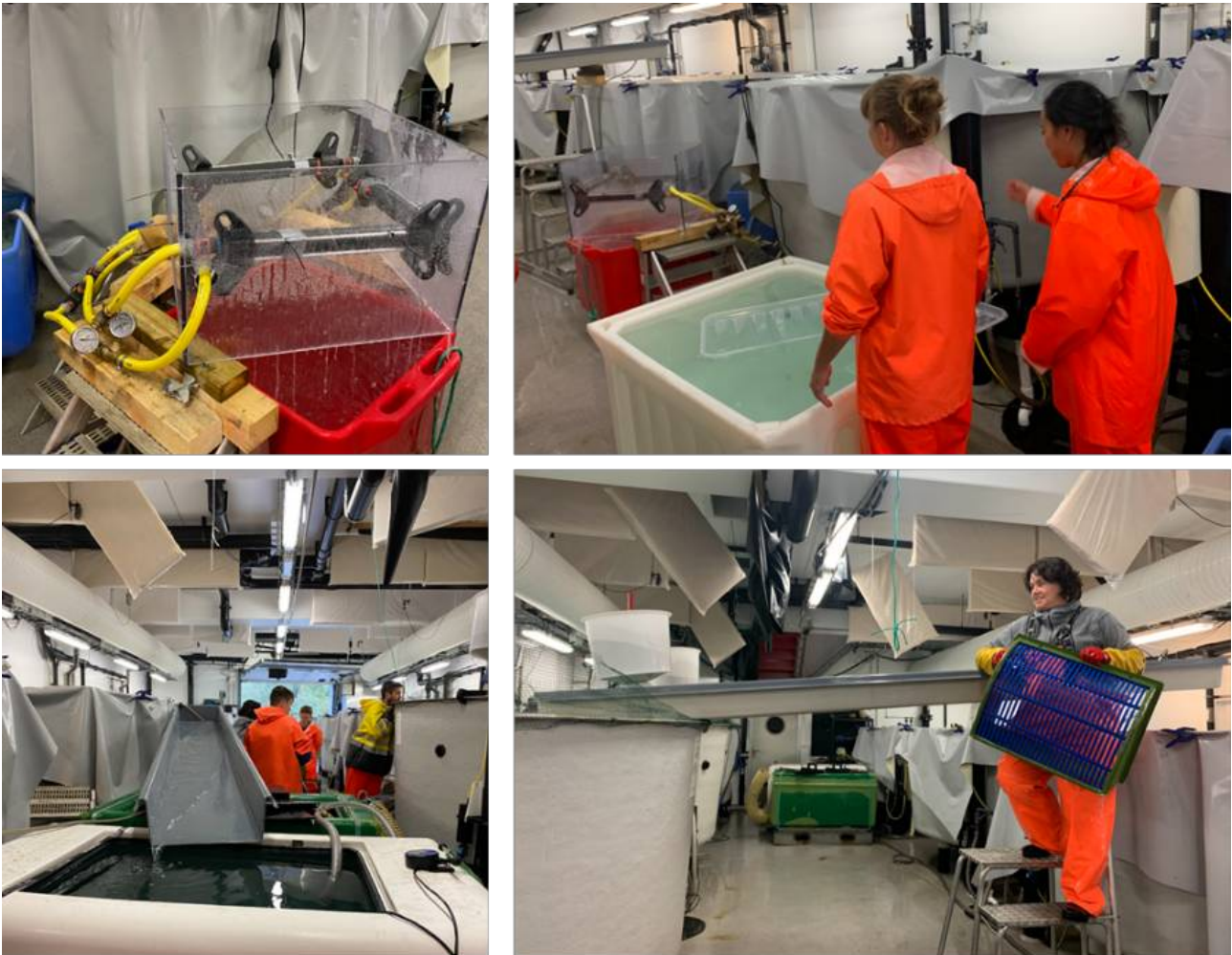
Fig. 1. Photos from the experimental setup. Upper left panel: the mechanical delousing device with nanometers for each input hose. Upper right panel: thermal treatments were applied in a 1000L transport tank. Lower left panel: half of the fish were placed in a run leading to a holding tank, before being transferred back into the experimental tank. Lower right panel: the latter half of fish were released into the run leading directly back into the experimental tank. Also shown is the blue 'basket' that held fish during transfer and thermal treatments.
