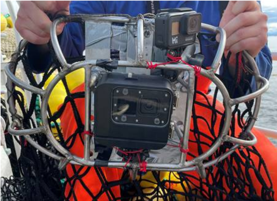
Figure 6: Steel frame with GoPro cameras fixed to the inside of the netting in the channel.
