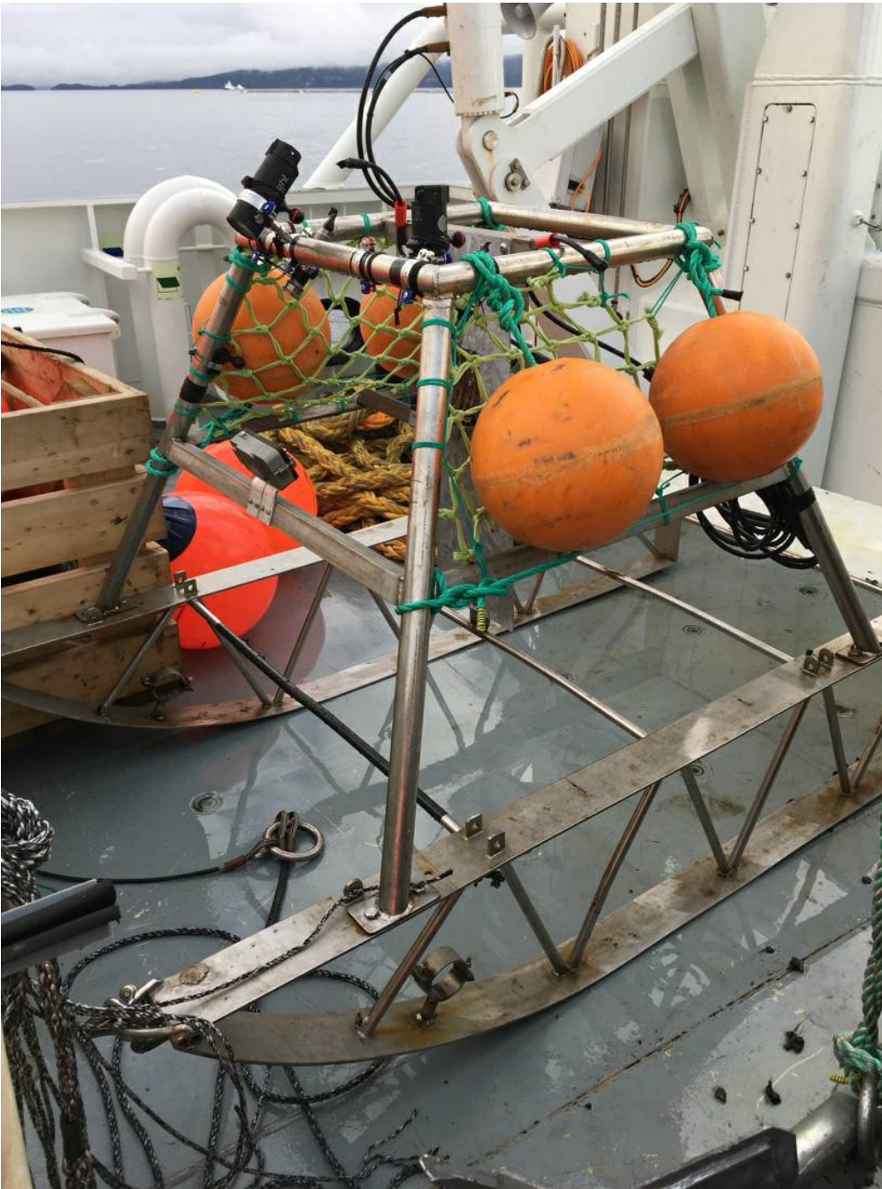
Figure 6: The video sled used for counting Nephrops burrows in the bottom sediment in the 2023 survey in Vestlandet. The two cameras (black) are mounted on top of the sled, one facing forward and one facing perpendicular to the sea floor.
